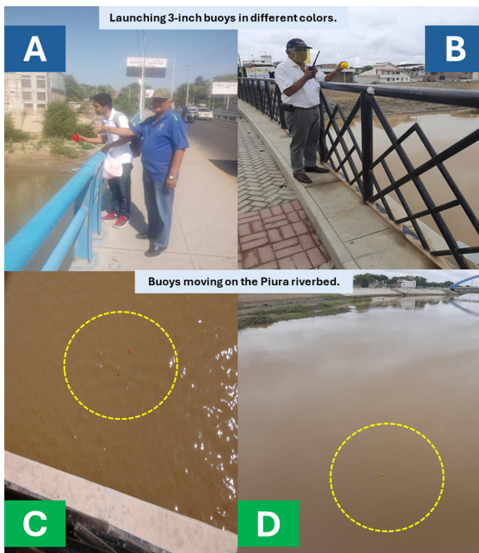
Figure 3. Launching and displacement of 3-inch buoys in the Piura riverbed Source: Authors, 2025.
